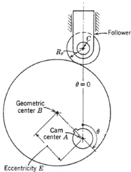
Write a spread sheet or a computer program, e.g. Matlab, to tabulate and plot the characteristics of the follower motion for one complete revolution of the cam, starting from its lowest position.
