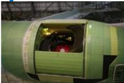
A view through the partially open telescope cavity door showing the aperture assembly (brown), telescope assembly structure (black) and cover over the primary mirror (red). February 3, 2006
