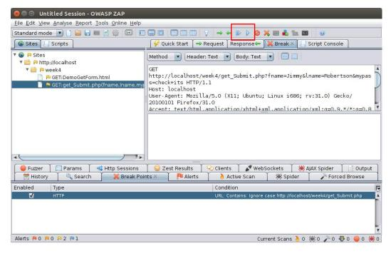
This is where the person-in-the-loop analysis and discovery takes place. Manipulating the data sent into the applications provides insight into the vulnerabilities of the application. For example, you may discover that sending in a null password allows access to the system. You may also discover providing an admin username and brute force password guess may provide additional system privileges.
