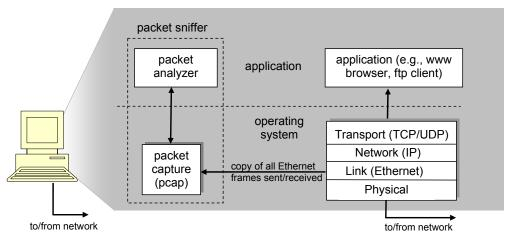
Figure 1: Packet sniffer structure
