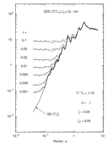
amplitudes of SDC tend toward a constant. For these short periods, the peak relative displacement of the columns is dominated by  $(1 + \delta)v_{\max}\tau$  and the peak shear forces in the first-story columns will result from this pseudo-static deformation caused by differential motions.
