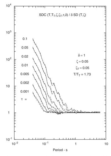
Fig. 7. Ratio of the new relative displacement spectra for columns and the old relative displacement spectra, SDC / $\delta$ SD, both shown in Fig. 6.
