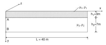
Fig. 10. Continuous two-dimensional analog of the models shown in Fig. 1a and 2, represented here by a "soft" layer ( $\mu_2$ ,  $\rho_2$ ,  $h_2 = 7$  m), corresponding to the first story columns, and a "hard" layer ( $\mu_1$ ,  $\rho_1$ ,  $h_1 = 3$  m), representing the upper part(s) of the structure.
