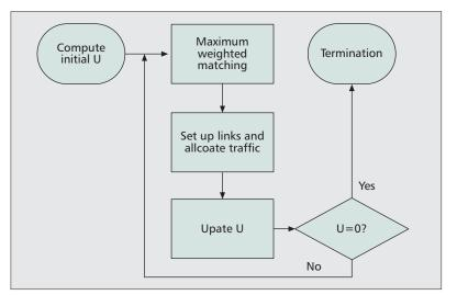
Figure 4. The flow chart of the heuristic algorithm.
