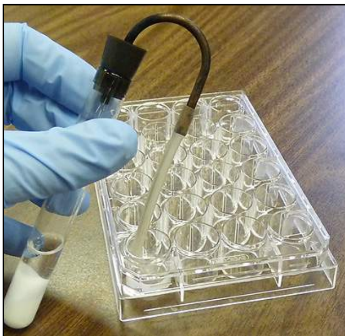
Figure 9. Hooked gas assembly in the limewater well.
