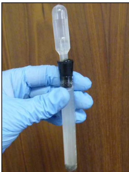
Figure 4. Gas generation tube.
