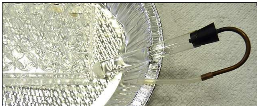
Figure 10. The test tube + gas assembly resting against the well plate.
