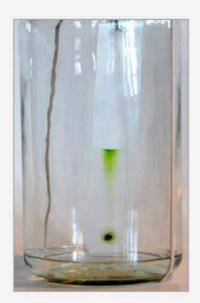
P. Attach the prepared chromatography strips to the paper clips. The strips should hang so that only the extreme end of the chromatography strip touches the solvent (acetone). DO NOT ALLOW THE ORIGIN LINE TO TOUCH THE SOLVENT.
