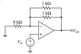
Solve for the gain,  $V_{\text{out}}/V_{\text{in}}$ , of the circuit above.
