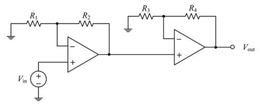
Which resistor values result in a circuit gain,  $V_{\text{out}}/V_{\text{in}}$ , of +5000 V/V?
