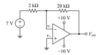
The op amp in the above circuit is ideal and has a saturation voltage of  $\pm 10$  V. Solve for the voltage,  $\nu_-$ , at the inverting input terminal.
