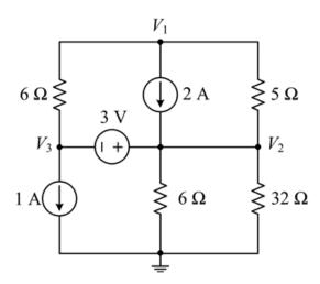
The supernode used to solve this circuit is located between which two nodes?
