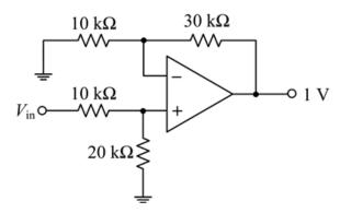
Which of the following input voltage values produce 1V at the op-amp output? Assume that the op-amp is ideal and is operating in its linear region.
