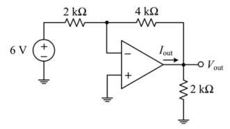
Determine the power supplied by the op-amp in the circuit above. Assume that the op-amp is ideal and is operating in its linear region.
