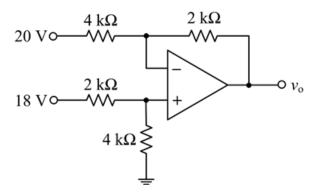
Solve for the value of  $v_0$  in the circuit above.
