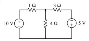
Solve for the voltage drop across the 4 ohm resistor.
