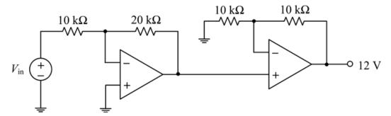
Solve for the value of  $V_{\rm in}$  needed to produce 12 V at the output.
