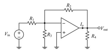
Which resistor(s) affect(s) the gain Vout/Vin?
