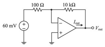
Determine the power supplied by the op-amp in the circuit above. Assume that the op-amp is ideal and is operating in its linear region.
