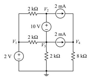
Solve for the voltages  $V_2$  and  $V_3$  in the above circuit.
