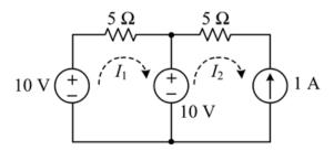
Solve for the currents  $I_1$  and  $I_2$  in the above circuit.
