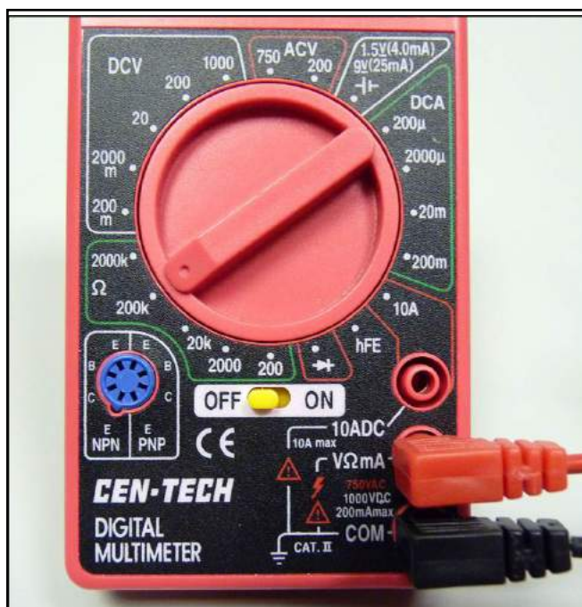
Figure 6. Multimeter with black and red cables. Note that the dial is set to 200k in the \Omega section.
