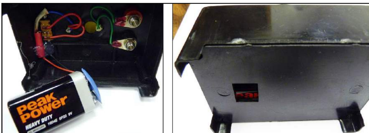
Figure 9. A. Battery connected. B. Bottom cover snapped into colorimeter.
