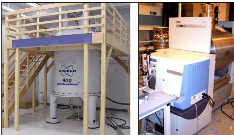
Figure 2. NMR and Mass Spectrometry. A. 900 MHz NMR spectrometer. © Charlesy B. Mass spectrometer. © Mkotl
